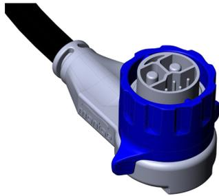
1. The connector at the end of motor cable (that plugs into the battery) can become contaminated with debris. Clear any debris from inside and around the contact pins by using light air pressure (blowing or using a light brush). Never place any conductive items into the pin area, taking care not to apply too much force that might damage or bend the pins.
